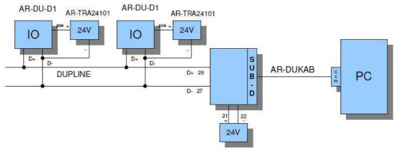
Example of configuration for 1 master module: 3-wire
