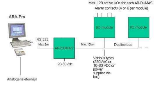
The modules are linked via a 2-wire bus cable. If modules are used that are supplied with power via a bus, the bus cable has three wires. This cable is not subject to any special requirements. The core's diameter is dependent on the maximum cable length. The following guideline can be used:
