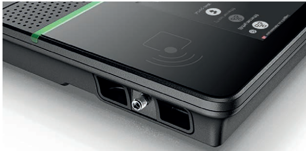
Antenna connector (SMA female). Maximum antenna gain: +8dBi
