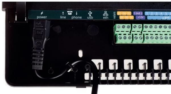
Placing the power cable in the S-shaped holder creates a strain relief. When replacing or using a power supply cord not included by Adésys the power supply cord must comply with IEC 60227-1.
