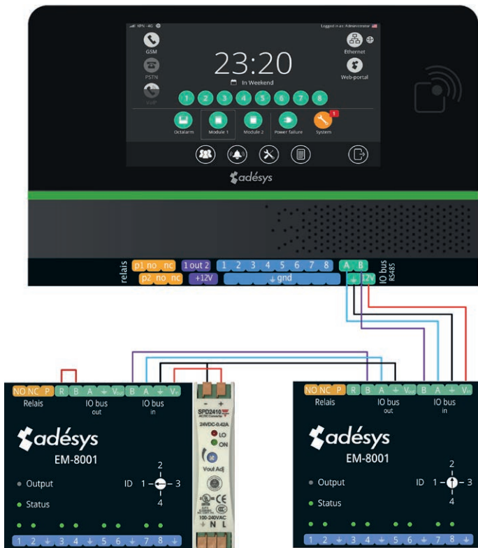
EM-8001 / Octalarm-Touch wiring diagram
