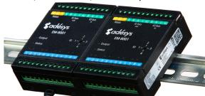
The EM-8001 can be used to extend the number of inputs on the Octalarm-Touch to 16 or even 24 (max. 2 modules per alarm). The EM-8001 is connected to the Octalarm-Touch via the I/O bus (RS485).
