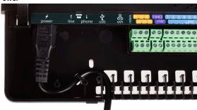
Insert the supplied power cable into the S-shaped holder; this creates a strain relief.
