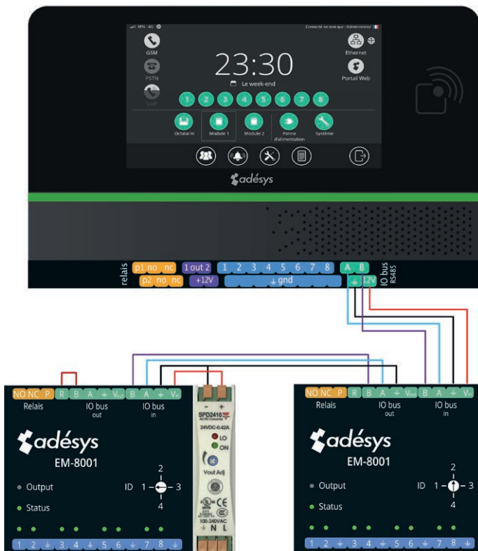
Schéma de raccordement EM-8001 / Octalarm-Touch
